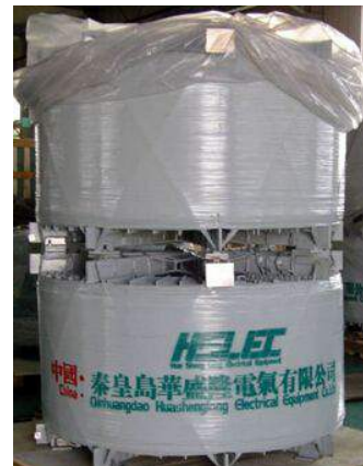
Air core shunt reactor
